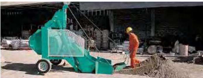
**CHARGEMENT DE LA BENNE PAR PELLE TRACTÉE (option)**
